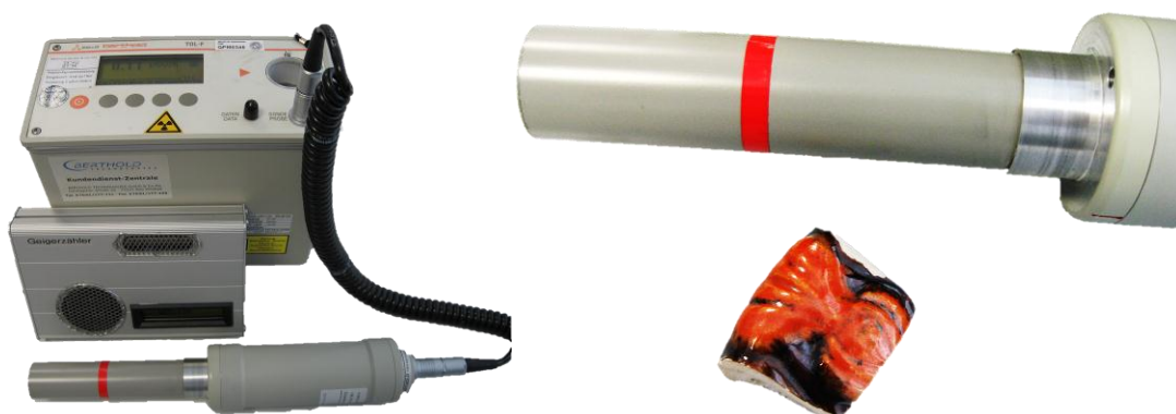
Figure 7: left, Geiger Counter Home-Made and professional equivalent dose meter Figure 8: right, The probe and a broken piece of ceramic plate
